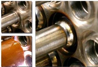
Orbital welding of element to tubesheet
